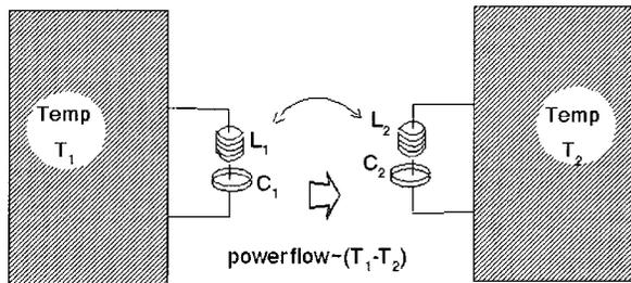
FIG. 2. Two coupled resonators at different temperatures.
